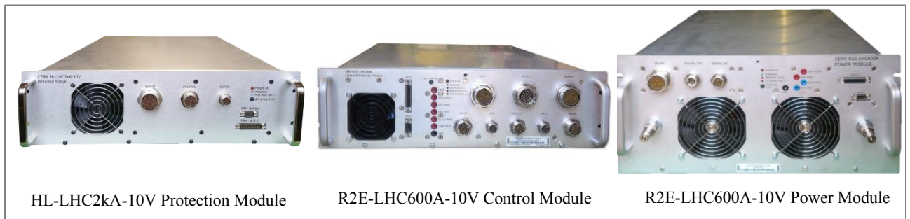
Figure 6B-2: Examples of 4-Q power converters modules that build up the full power converter.
